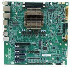
micro-ATX motherboard supports 14th Gen. Intel® mobile Meteor Lake-H on-board processor, DDR5, 2.5GbE LAN, M.2, USB 3.2, SATA 6Gb/s, HD Audio and RoHS
