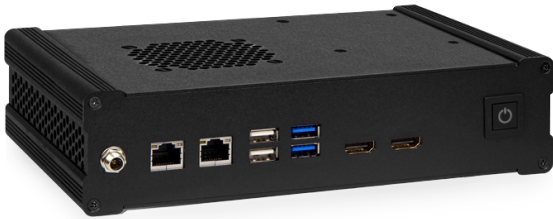
BRICK Chassis with WAFER-AL (SBC not included)
